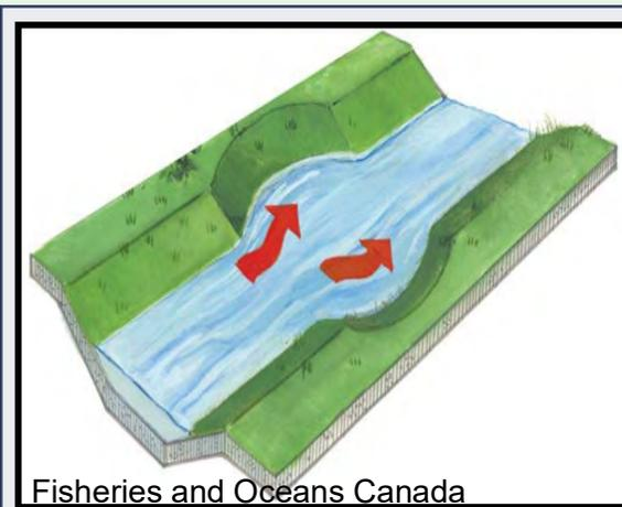
Plan view of an on-line sediment trap (left).
